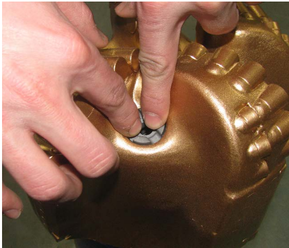
Figure 9. Hand Tighten Nozzle
