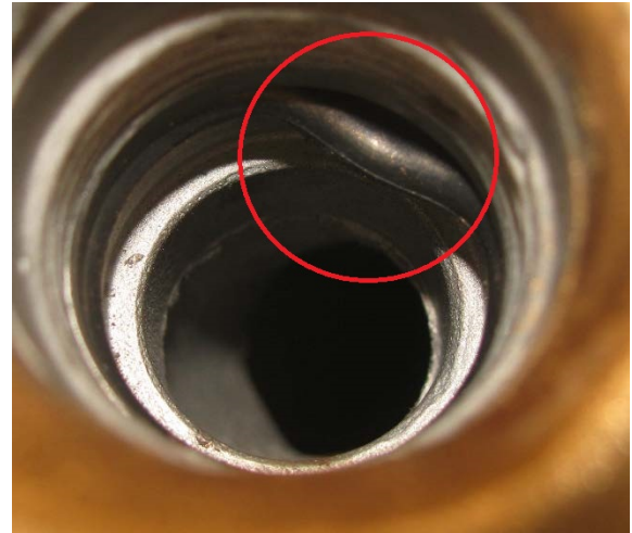
Figure 6. O-Ring Not Seated
