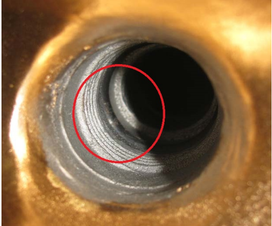
Figure 4. Inspect Nozzle O-Ring
