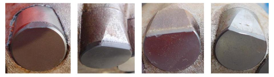
FC – Flat Crested Wear can be classified as WT – Worn Cutter. However, FC - Flat Crested Wear is suggested when wear is smooth and flat.
